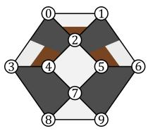
In this figure we see an example stabilizer code. Data qubits are indicated as white circles and are labelled by numbers. Polygons represent checks. The coloring of the polygons indicate how the associated check acts on qubits it touches. When the check is white on a qubit, the check acts as Z. When black, X. When brown, Y.
