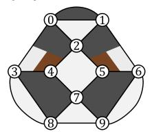
We seemly failed to create a higher distance code; however, we can persevere by removing a higher-weight stabilizer generator. If we remove the check that acts like Pauli Z on qubits 7, 8, and 9, we will get the stabilizer code in:
